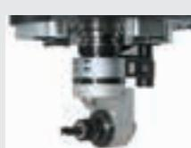
The maximum speed of the standard angle tool is 3000 rpm. The angle tool can be stored in the 30-tool and 60-tool magazines.
